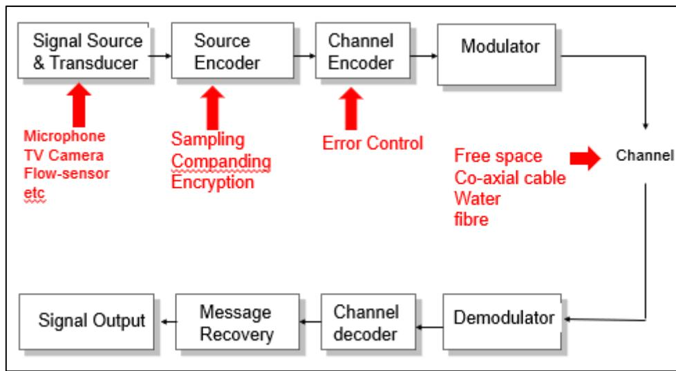
**Source Encoder:** Removes redundancy from the data (compression).
