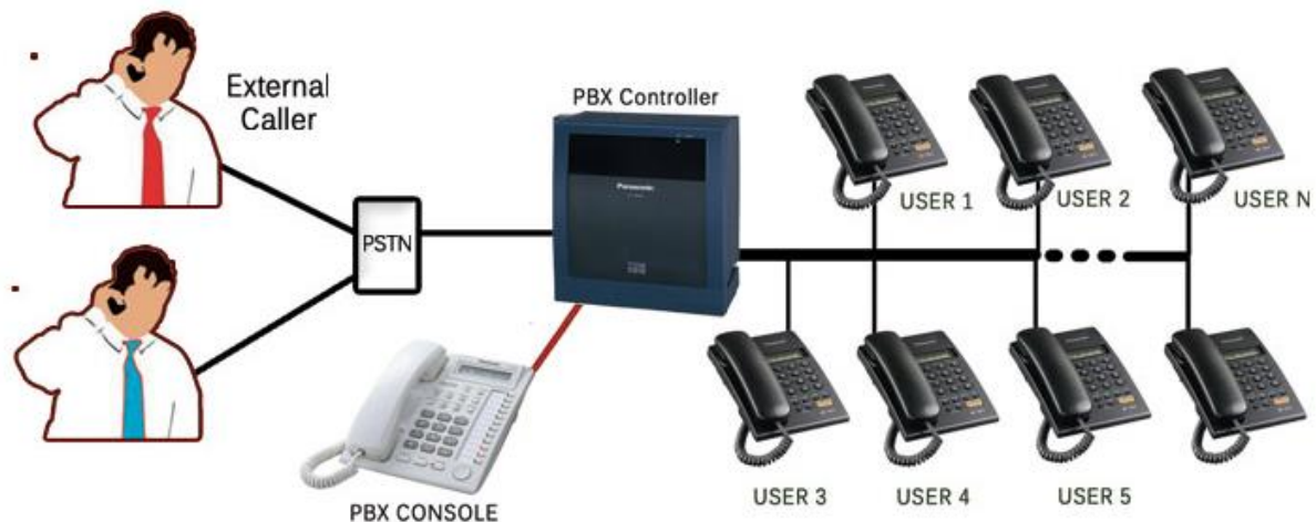
Figure 1. Functional units of a Private Automatic Branch Exchange (PABX)
